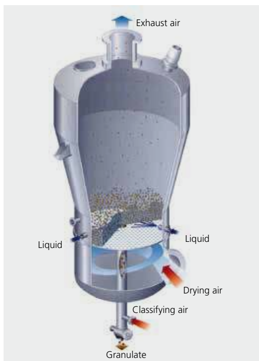
Continuous granulation dryer WS-GT with classifying product discharge
